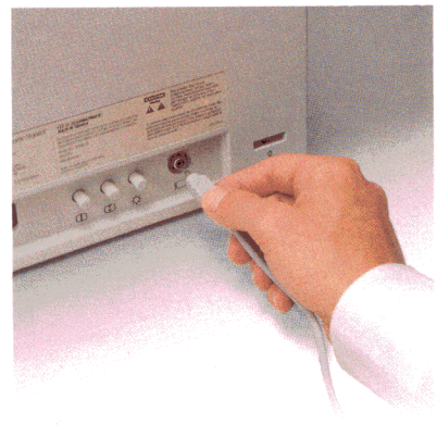
Figure 1-14 Plugging the monitor cable into the monitor
