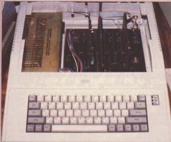
A look inside the Pravetz, the only II clone that features built-in slots like the Apple II.
