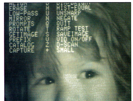
Composite monitor lets you see ImageWorks menus overlaid on digitized video output.
