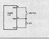
use IF...THEN statements such as the following to detect whether or not a switch connected to this pin is open
