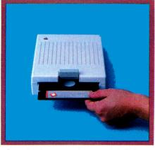
**Photo 2.** The optional external disk drive. It has a formatted capacity of 143K.
