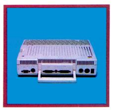
**Photo 1.** The back panel showing the ports through which the //c communicates with the world.
