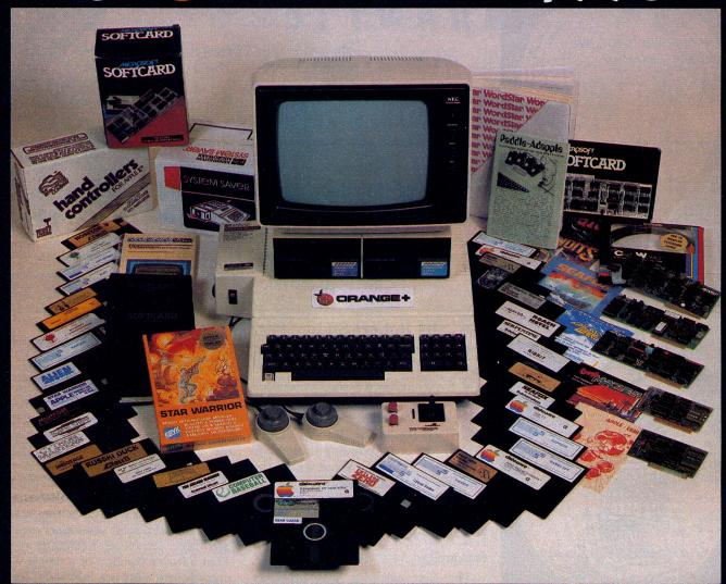
Finally, a dynamic powerful, practical personal computer that is fully Franklin Ace 1000 and Apple. Il compatible, yet, lower in price than the competition. Uses existing available software. The "ORANGE+" is the pacesetter of the future, with a switchable 110-220 volt power supply, upper and lower case with lower case locking key, enhanced audio and color functions, 8 slot motherboard, game port, fully socketed I.C. board, a 3 ROM operating system, 48K ram, fully expandible.
