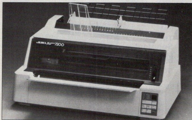
The Juki 7200, a 24-pin color dot-matrix printer
