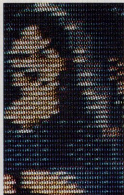
Figure 3: Screen photo of same portion of art from the Apple IIGS on a standard composite monitor
