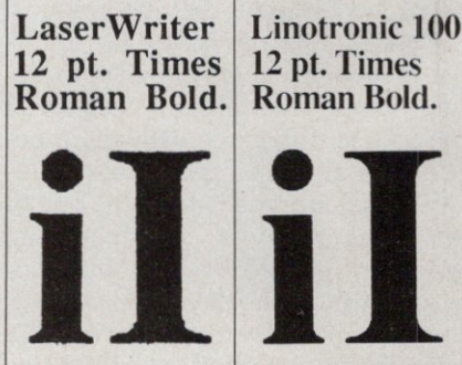
Figure 1: A comparison between output from a laser printer (left) and a Linotronic typesetter (right). Lower- and uppercase letter I's are 24-point type enlarged 400%.
