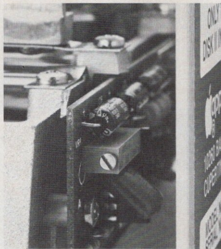
Figure 7: The disk-drive speed-adjustment screw is located inside the disk drive on the right side, in the rear. Using a speed-diagnostic program to display the speed of your drive, adjust the screw until the speed of the drive is within tolerance.
