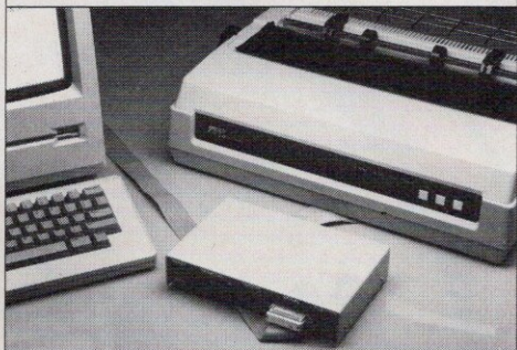
The MACpac letter-quality, daisy-wheel-printer system includes the TTX 1014 printer, the MACbuf 64K buffer, and a printer/buffer cable.
