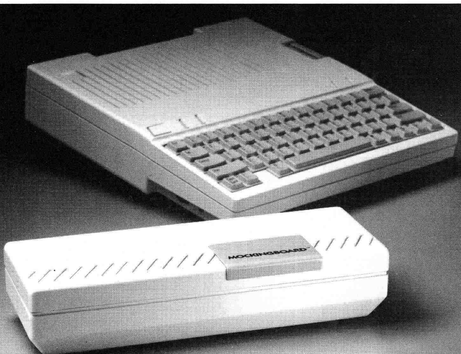
Mockingboard IIc provides synthesized speech, music, and sound effects for the Apple IIc.
