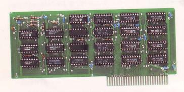
• 16K memory expansion card for the Apple II and II+ fully compatible with Applesoft, CP/M and Pascal. Plugs into slot 0.
