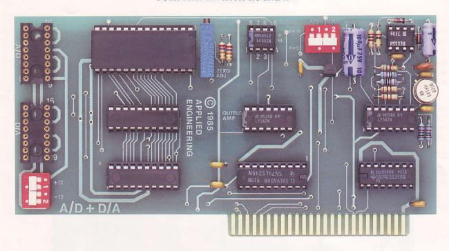
Commercial, industrial, and scientific data acquisition and control functions are now practical with Applied Engineering's A/D + D/A card.
