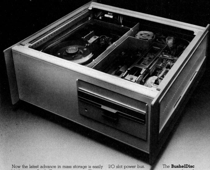
added to your Apple II computer system. The new 9670-110A BushelDisc® from Creative Micro Systems is a magnetic disc storage module that provides 10 megabytes of fast, reliable Winchester storage and an integral 1 megabyte flexible diskette backup channel. You can expand the system with additional drives for as much as 80 megabytes of on-line storage.
